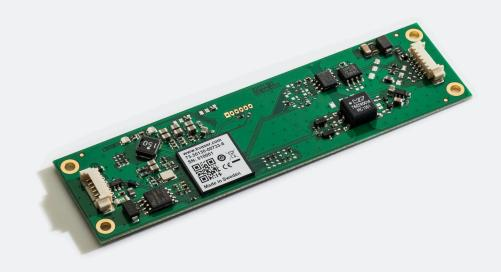
The Leaf Light v2 CB is the bare circuit board version of Kvaser's popular Leaf Light v2 interface - a single-channel, high speed, USBto-CANbus interface. Having made its name as the workhorse of USB to CAN interfaces, Kvaser's Leaf Light product series provides reliable, low cost connection to the PC.
