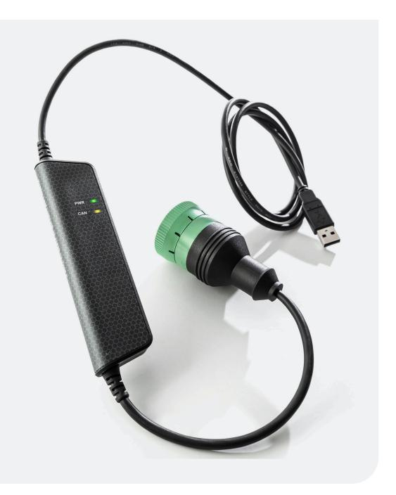
The Kvaser Leaf Light HS v2 J1939-13 Type II provides a simple way of connecting a PC with the on-board computer of any J1939 compliant vehicle or industrial system. Get diagnostic data by means of its USB 2.0 connector and a 9-pin J1939-13 (Type II) compliant CAN connector, which is colour-coded in green and supports either 250 Kbps or 500 Kbps vehicle networks.
