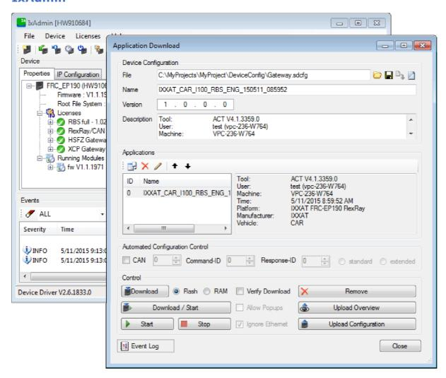
Administration tool for the embedded platform which is connected to the device via USB, Ethernet or Wi-Fi.
